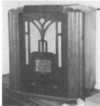
CORONADO - A battery operated radio, it was made sometime in the 1920's, I think. Tubes include 1-A-6, 30, 32, 33 and 34. (From the collection dubbed "Tony's Old Ladies.") (Anthony B. Parks - Franklin Grove, IL)
