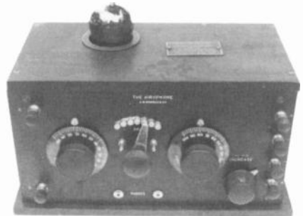
CORONADO - A battery operated radio, it was made sometime in the 1920's, I think. Tubes include 1-A-6, 30, 32, 33 and 34. (From the collection dubbed "Tony's Old Ladies.") (Anthony B. Parks - Franklin Grove, IL)
