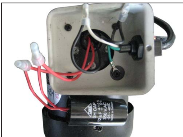
Figure 102. G1079R feed motor connections and run capacitor.
