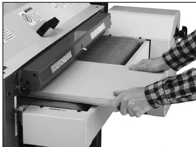
Figure 67. Example of using D3003 PRO-STIK® Cleaning Pad to clean sandpaper.
