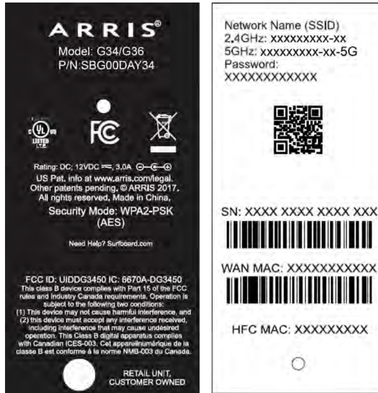
Figure 3: Sample G34/G36 Wi-Fi cable modem label
