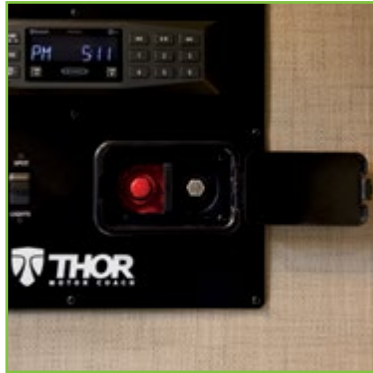
Garage Jumpstart Charging Center
