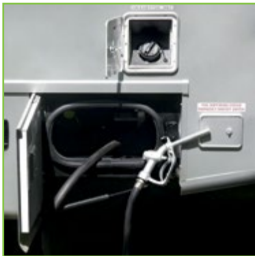
Remote Fuel Filling Station with Auxiliary Fuel Tank, Pump and Nozzle
