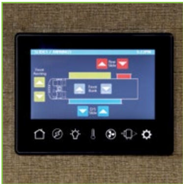
Multiplex Wiring Control System with 7" Touchscreen
