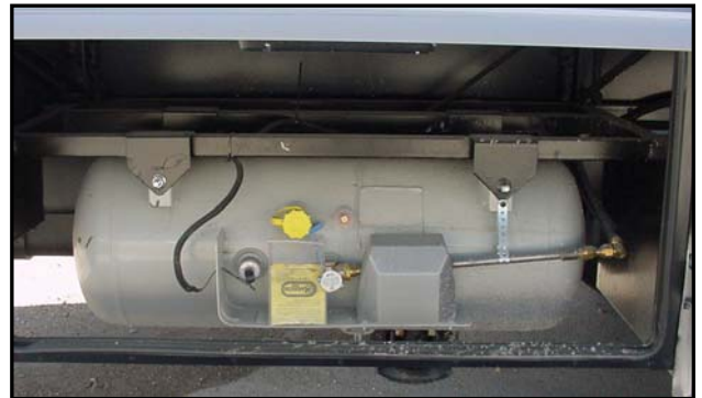
Figure 3-4. Liquid Propane Tank
