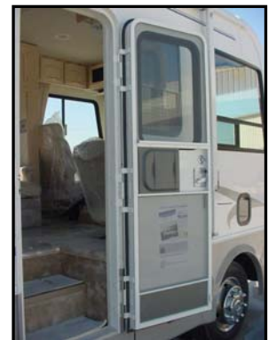
Figure 13-6. Front Door & Screen Door
