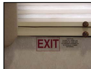
Figure 2-7. Emergency Exit Window
