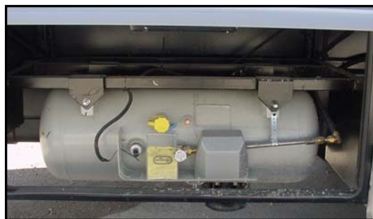
Figure 2-2. Liquid Propane Tank
