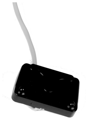
Photo-Eye Module Separated from Holder
