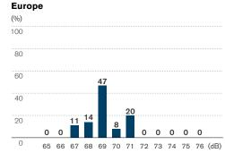
Noise emissions are shown by the noise produced by the acceleration of vehicle in accordance with each national regulation. Only complete, built-up imported models are shown for China data.
