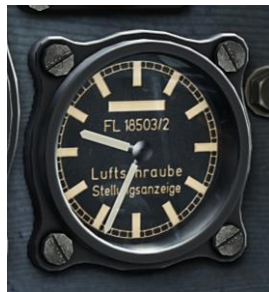
Figure 80: Prop Pitch Indicator in 9:34 Position
