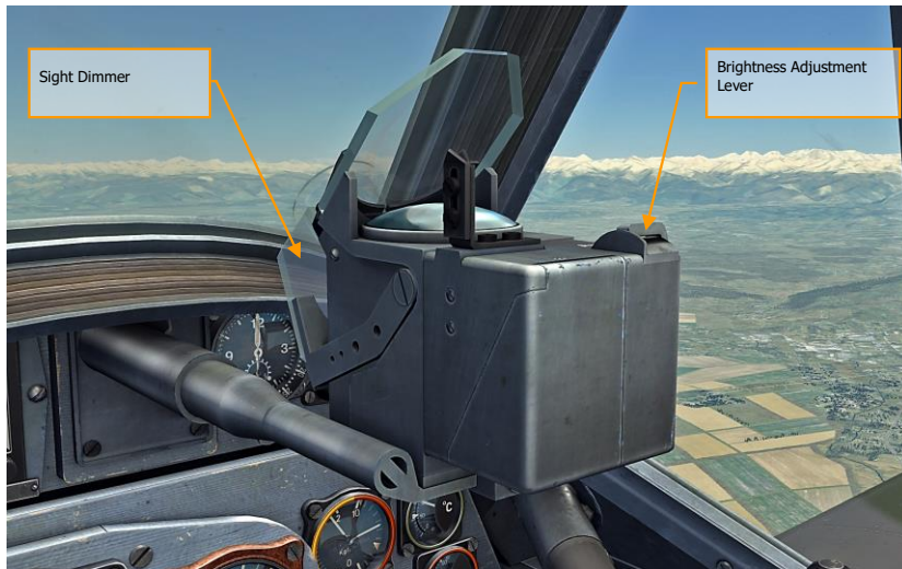
Figure 61: Revi 16B Gunsight in unfolded combat position
