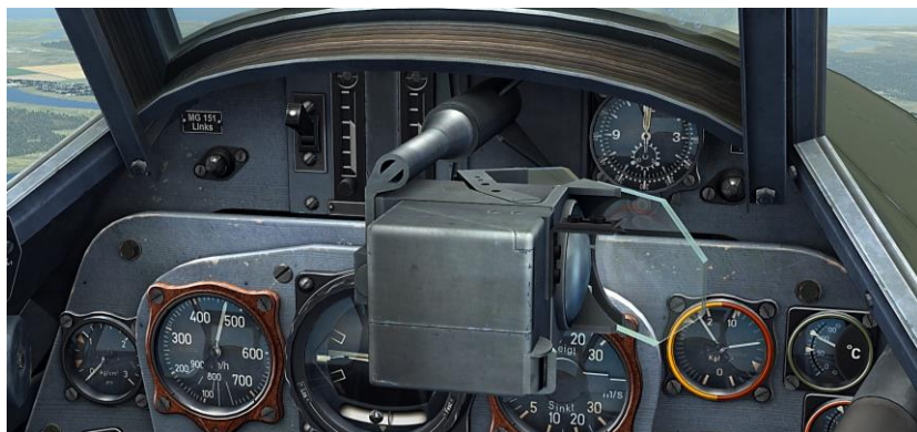
Figure 63: Revi 16B Gunsight in folded position
