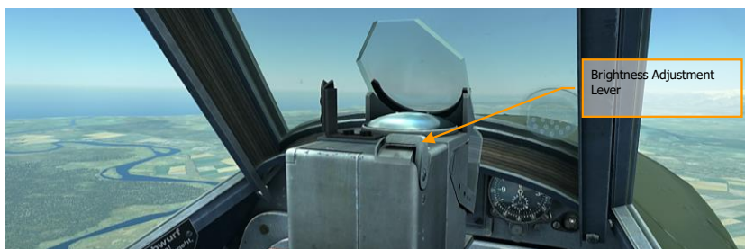
Figure 62: Gunsight's Brightness Adjustment Lever
