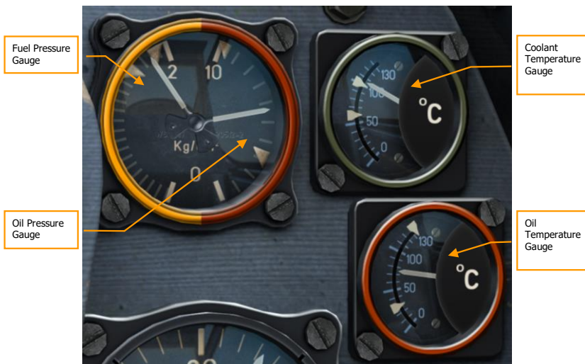
Figure 78: Fuel and Oil Pressure Gauge, Coolant and Oil Temperature Gauges
