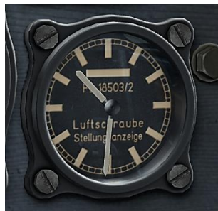
Figure 33: Propeller Pitch Position Indicator showing 10:30 or 38 degrees prop pitch
