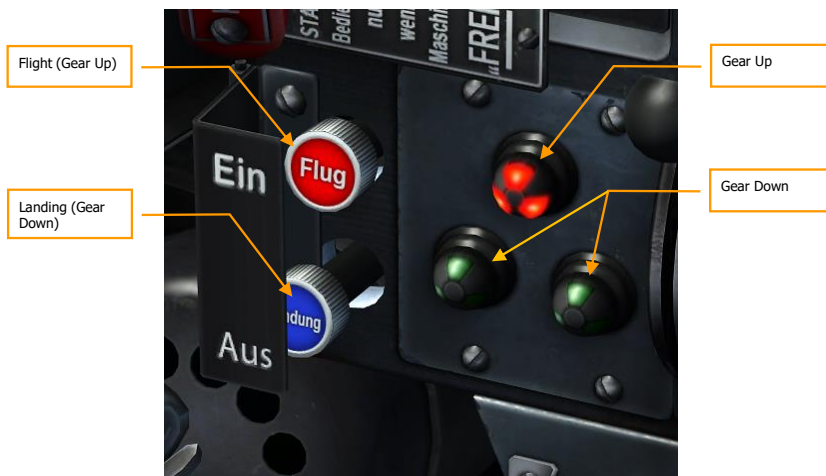
Figure 72: Landing Gear Controls and Landing Gear Position Indicator
