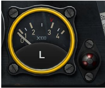
Figure 36: Fuel Contents Gauge and Fuel Warning light
