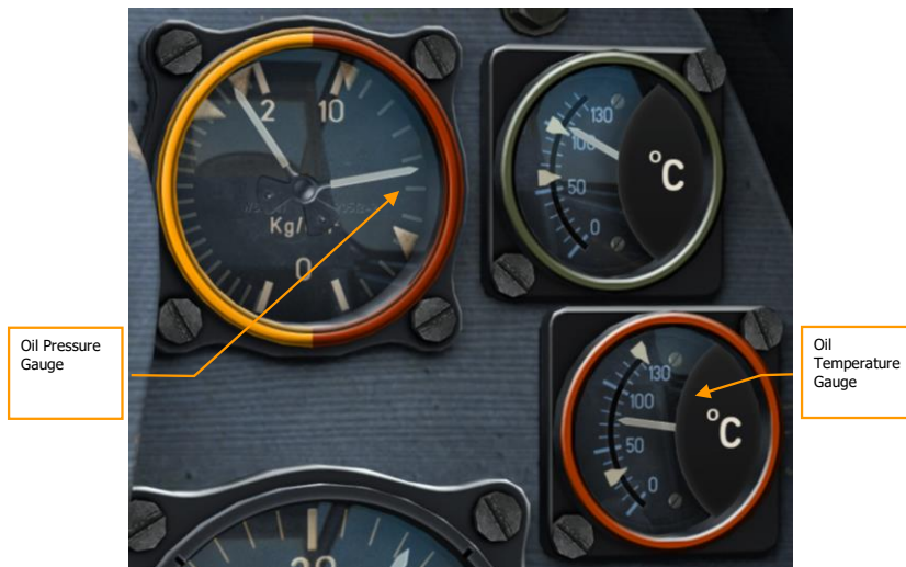
Figure 42: Oil Pressure (right) and Oil Temperature Gauges
