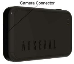
i. Used to connect Arsenal 2 Pro to the Camera with the Coiled USB Cable.
