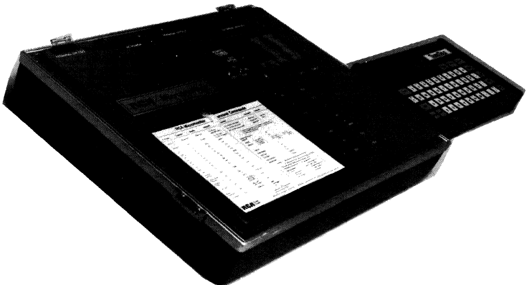
Fig. 7 - RCA COSMAC Micromonitor CDP18S030A.
