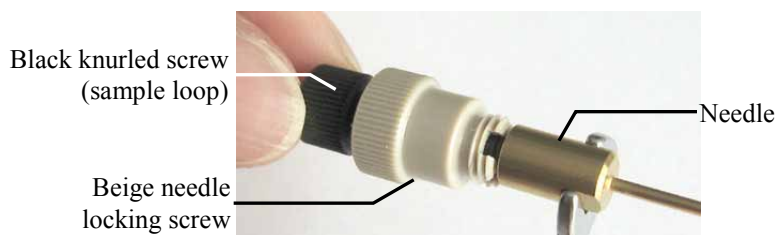
Fig. 43: Disconnecting the needle from the sample loop
