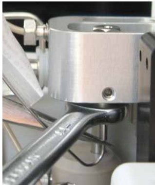
Fig. 76: Tightening the needle seat capillary
