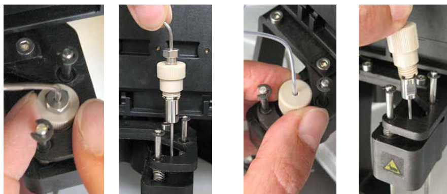
Fig. 45: Removing the needle from the needle holder (left: WPS-3000SL Semiprep; right: WPS-3000TBSL Analytical)
