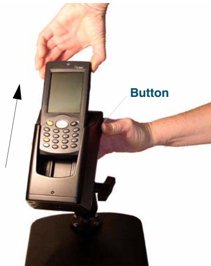
Figure 14. Removing the 4220 from the Dock
