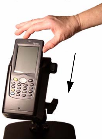
Figure 13. Inserting the 4220 into the Vehicle Dock
