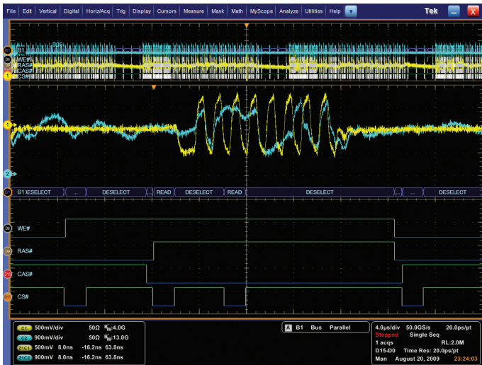
Figure 4. Bus qualified trigger of memory read cycle.
