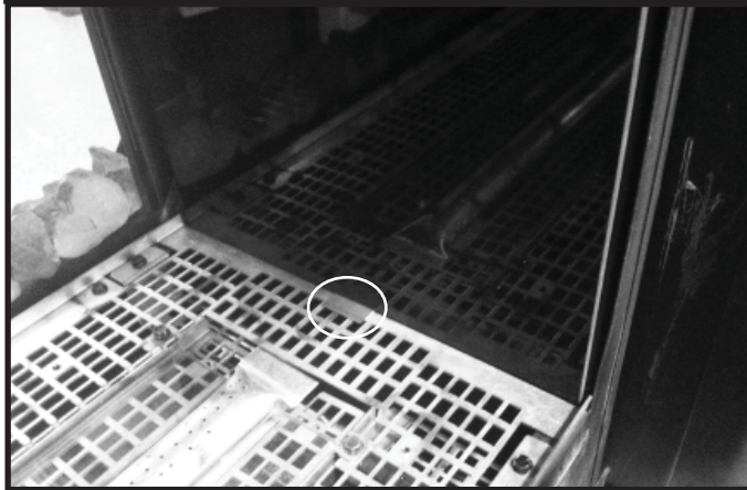
Figure 10.8 Position Glass Clip and Install Glass Panel
