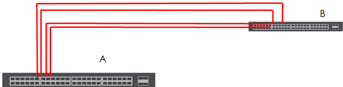
Figure 125 Trunking Example - Physical Connections
