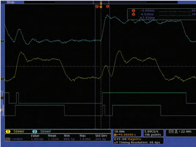
Figure 52. The MSO provides 16 integrated digital channels, enabling the ability to view and analyze time-correlated analog and digital signals. A high speed timing acquisition provides more resolution to reveal narrow events such as glitches.
