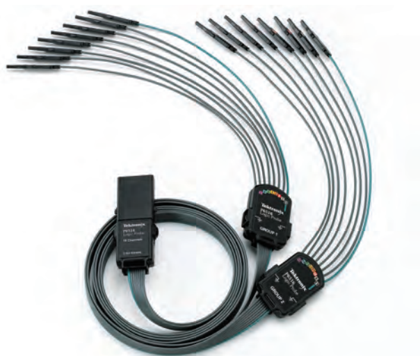
Figure 43. Logic probes for a mixed signal oscilloscope (MSO) simplify digital connectivity to your device.
