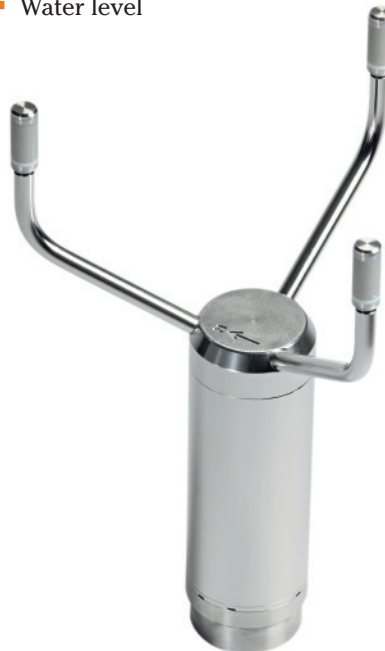
Vaisala WINDCAP® Ultrasonic Wind Sensor WMT700 is maintenance-free, with no moving parts, and the patented three-transducer layout provides accurate data in all wind directions.
