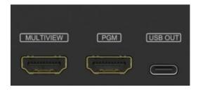
HVS0402U has 3 output interfaces. They are default as Multiview Out, PGM Out and USB Out. All the 3 outputs also can be defined as an AUX OUT from HDMI1, HDMI2, HDMI3, HDMI4, PVW, PGM, Clean PGM, Color Bar and Multiview out.
