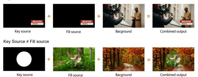
DSK button ON: DSK key shows on PVW.
