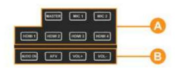
Part A is for selecting one audio to be configurated, including Master, MIC 1, MIC 2, HDMI 1, HDMI 2, HDMI 3 and HDMI 4.
