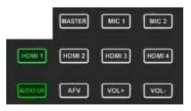
After pressing one Part A button, the indicator of button in Part B is on in green means the corresponding audio function is on. When the indicator is off means the corresponding function is off.
