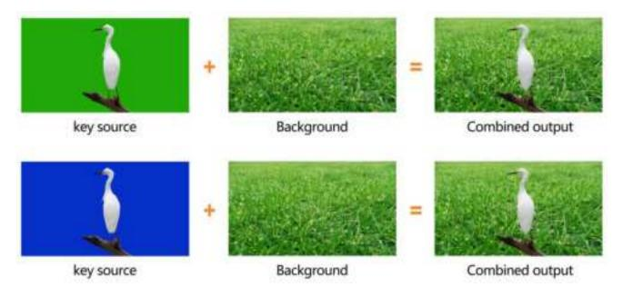
Turn on the CHROMA key button, press Menu knob and choose the Chroma to configure the effect of Chroma Key, including the key source, Key color, Clip, Gain, key Fetch and mask, etc., detailed parameters setting as below.
