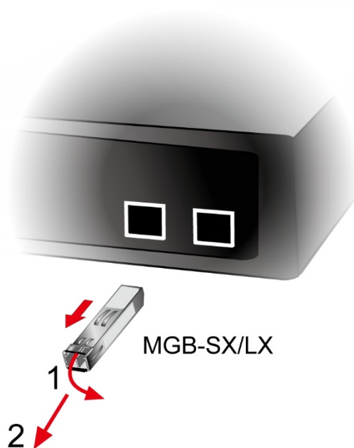
Figure 2-2-5: How to Pull Out the SFP/SFP+ Transceiver
