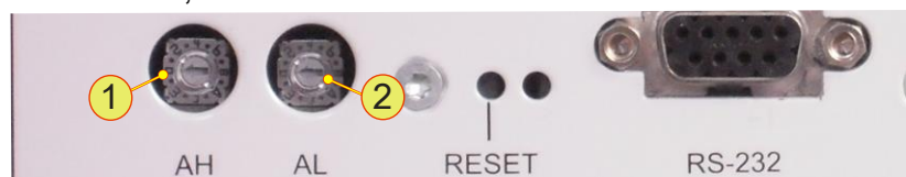
Fig. 32 Rotary switch AH -1- for the upper address range Rotary switch AL -2- for the lower address range
