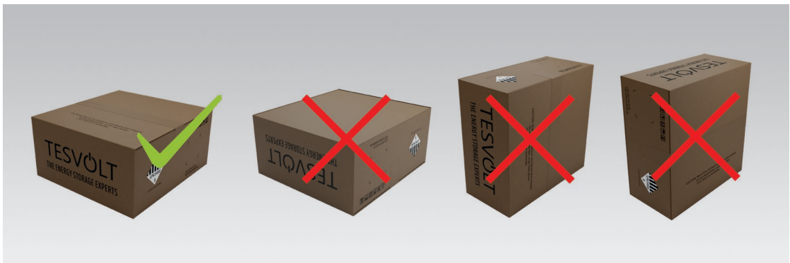
Abbildung 3.1 Permissible and impermissible storage positions of a packaged battery module
