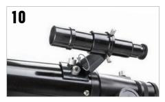
Locate the finderscope and remove plastic caps on front and back of lens. Orient the finderscope so that the longer lens is facing towards the front of the tube as shown here. Place finderscope over the posts on the tube and replace knurled nuts to secure.
