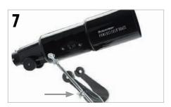
Locate the optical tube and insert the attached slow motion control rod into the hole on the mount.
