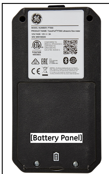
Figure 50: Battery Panel Location
