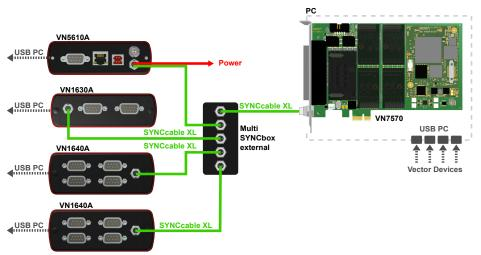
Figure 73: Example of a time synchronization with multiple devices
