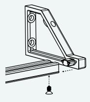
3. Carefully remove the decorative caps and the four screws on the front of the VN device.
