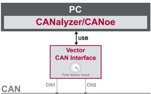
Figure 69: Common time stamp clock for each channel
