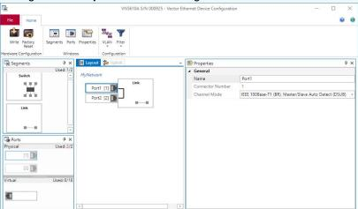
8. Click the **Write** icon in the tool bar. The configuration is now persistently written to the VN5000 interface. The configuration will be recovered in **Vector Ethernet Device Config** when opening it again.
