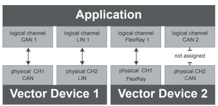
Figure 58: Concept of channel assignments
