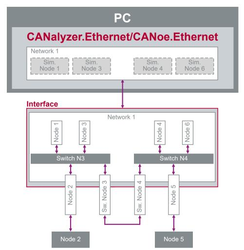
Figure 66: Simulation setup of the device driver from version 11.2
