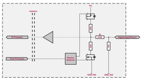
Figure 27: Digital input /output
