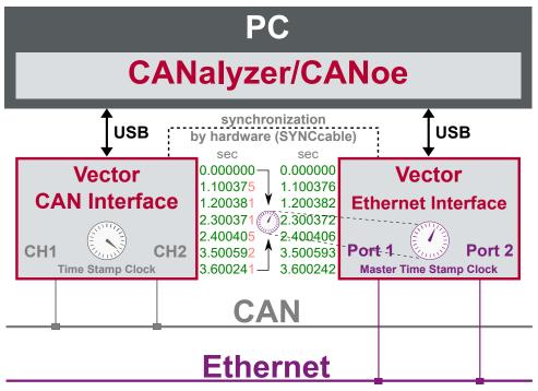
Figure 75: Time stamps are synchronized to the master clock
