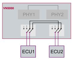
Figure 55: Bypass active, Vector Ethernet Network Interface is switched off
