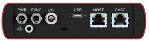
Figure 15: Connectors on the USB side
