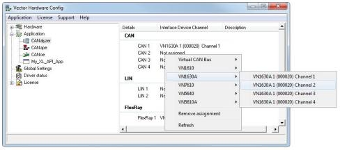
Figure 59: Channel assignment in Vector Hardware Config
