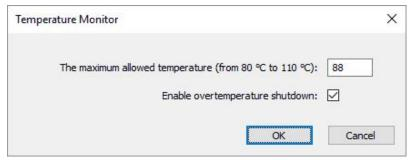
Figure 18: Setting limit for shutdown
