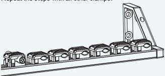
8. Finally, lead the individual cables through the clamps and tighten the individual clamps depending on the cable (Torx 10).
