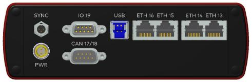
Figure 26: Connectors on the USB side
