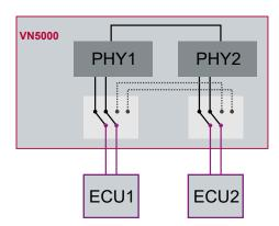
Figure 54: Bypass inactive, Vector Ethernet Network Interface tunnels ECUs
