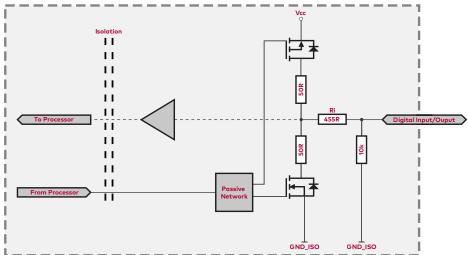
Figure 11: Digital input /output
