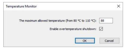
Figure 24: Setting limit for shutdown
