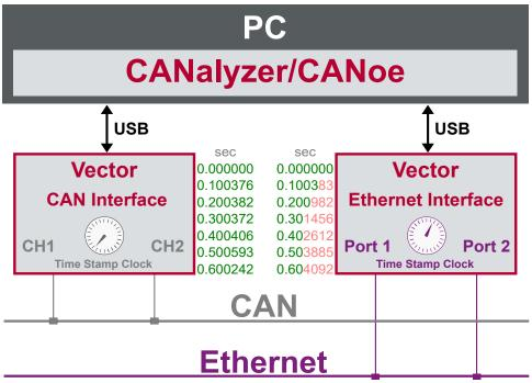
Figure 70: Example of unsynchronized network interfaces. Independent time stamps drift apart
