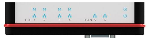
Figure 16: Top LEDs on VN5620
