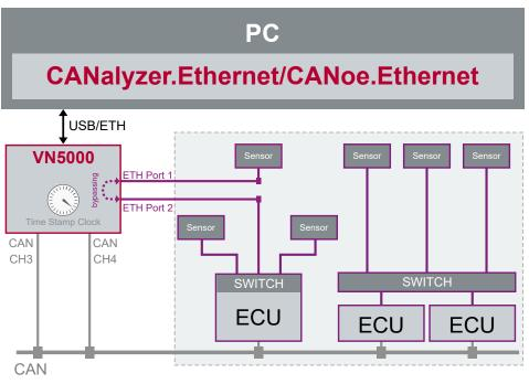
Figure 2: Extended measuring setup
