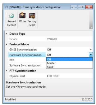
Figure 76: Configuring hardware synchronization
