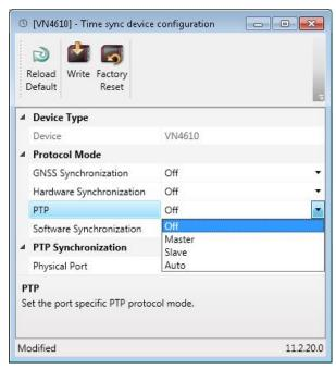
Figure 78: Configuring PTP synchronization
