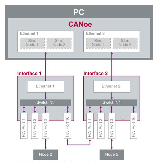
Figure 65: Simulation setup of the device driver before version 11.2
