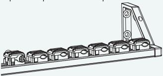
8. Finally, lead the individual cables through the clamps and tighten the individual clamps depending on the cable (Torx 10).
