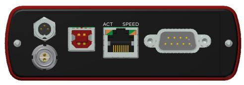
Figure 10: Connectors on the USB side
