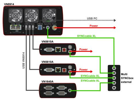
Figure 74: Example of a time synchronization with VN8914 and additional devices
