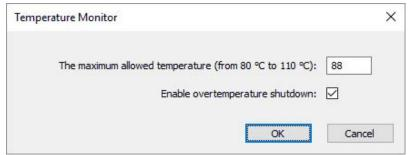
Figure 53: Setting limit for shutdown
