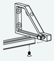
3. Carefully remove the decorative caps and the four screws on the front of the VN device.
