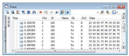
Figure 68: Time stamps of two CAN channels in CANalyzer
