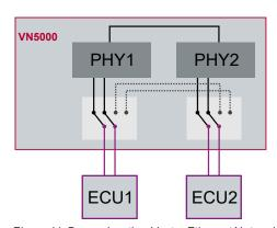
Figure 41: Bypass inactive, Vector Ethernet Network Interface tunnels ECUs
