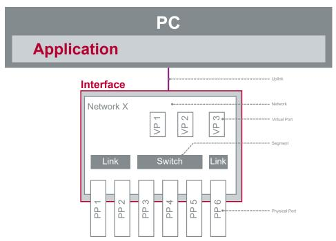
Figure 67: Simulation setup of the device driver from version 11.2
