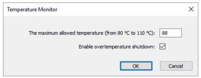
Figure 40: Setting limit for shutdown
