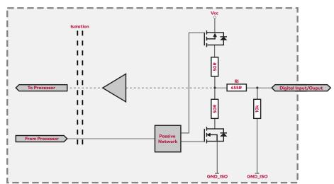
Figure 47: Digital input /output
