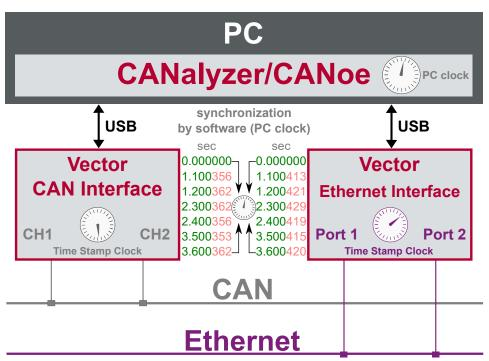
Figure 71: Time stamps of devices are synchronized to the PC clock
