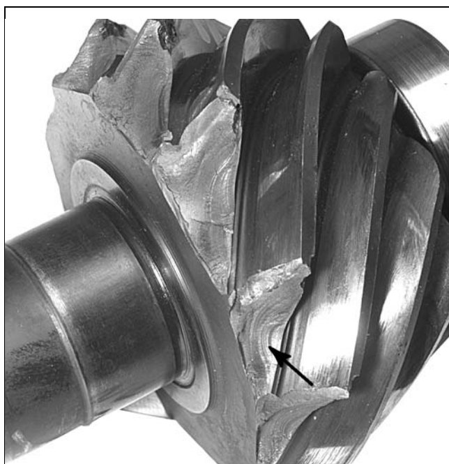
TEETH BROKEN DUE TO FATIGUE AT HEEL END
