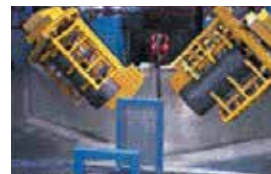
Tanks are then rotated further, allowing the excess PermaGlas to drain from the tank.
