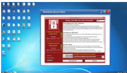
Ransomware is safely contained within a disposable micro-VM, easily clicked away when the user closes the window.
