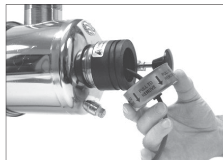
Step 2 – Remove End Cap
