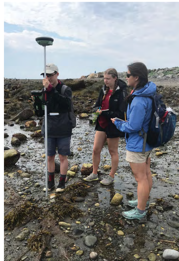
Students recording precision elevations of intertidal habitat zones using RTK-GPS.
