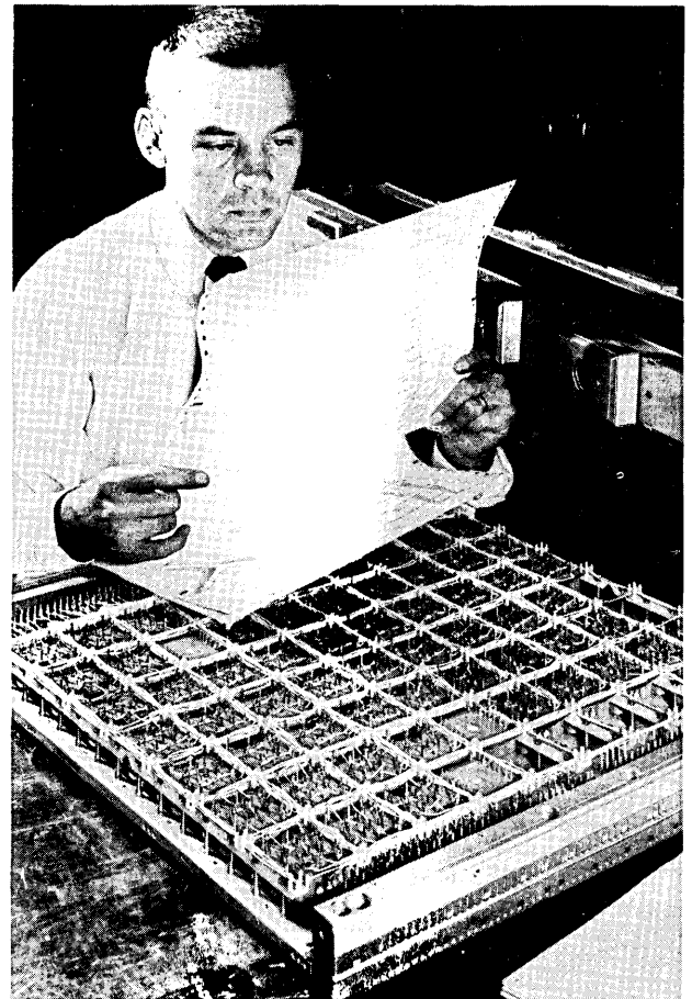
— A Bell Laboratories' engineer at Whippany, N.J., checks design information for the first computer built from complete information furnished by another computer. A subassembly of the computer is on the table. The computer will be used with the target-track radar for the Army's NIKE-ZEUS anti-missile defense system. --
