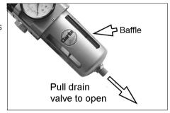
With use, the filter will become sufficiently blocked that the air throughput can become severely diminished. It should be removed and cleaned as follows:
