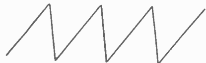
FIG. 127.—Saw-tooth waveform of voltage for X deflection as a function of time.
