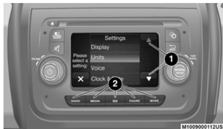
Uconnect 3/3 NAV With 5-inch Display Buttons On The Touchscreen And Buttons On The Faceplate
