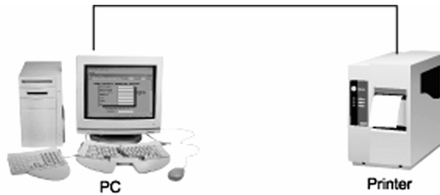
Figure 2-A: Connection Type 1 “Local” – Direct Connection: PC to Printer
