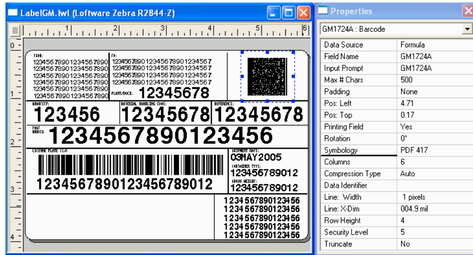
Figure 7-1: GM label 1724-A created using the GM Bar Code Template and Wizard
