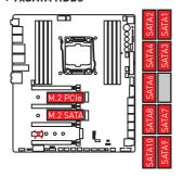
2xM.2 PCIe SSDs + 4xSATA HDDs + 1xPCI\_E4 Device
