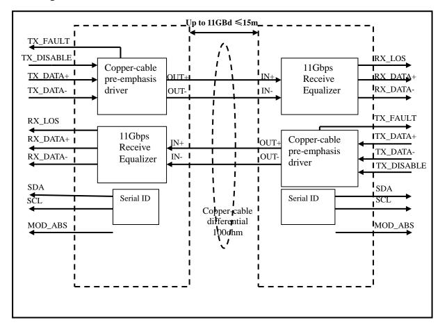
Active cable assembly has signal amplification and equalization in the assembly. Active copper assemblies are typically used in host systems that do not employ EDC. Active SFP+ cable assemblies also incorporate Rx LOS and Tx Disable features.
