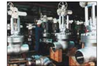
Full bore parallel slide gate valves in low carbon steel for a nuclear power plant.
