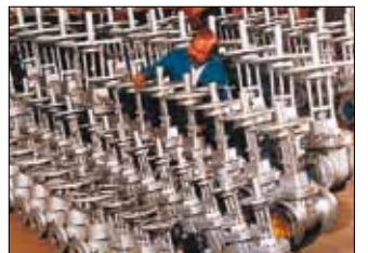
Volume production of gate valves for low/medium general purpose industrial duties.
