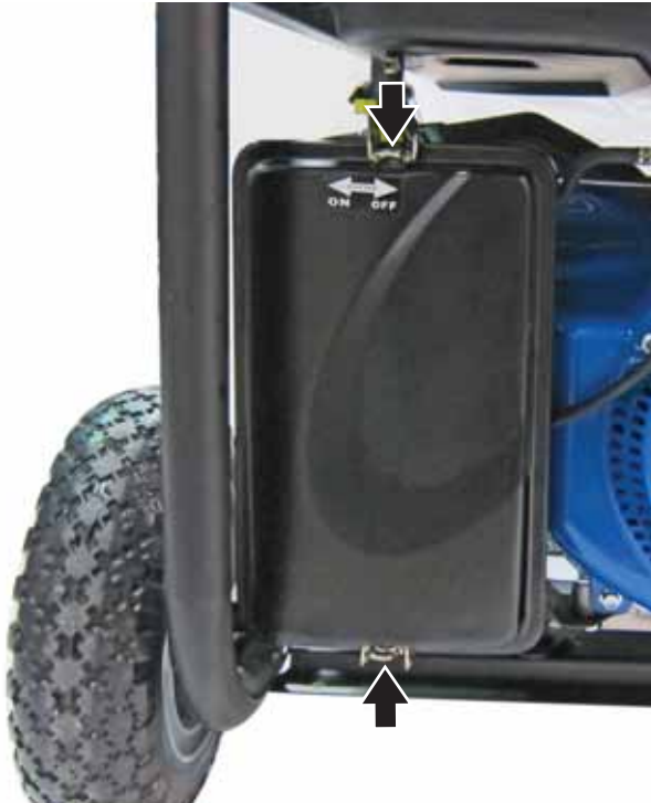
Figure 7-13 – Installation of Air Filter Cover
