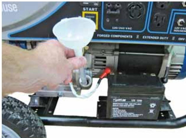
Figure 7-5 – Adding Engine Oil
