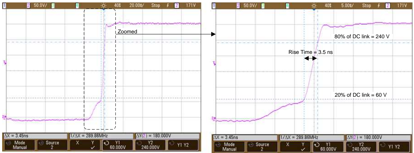
Figure 27. Turn-off Transition at 1.6 A
