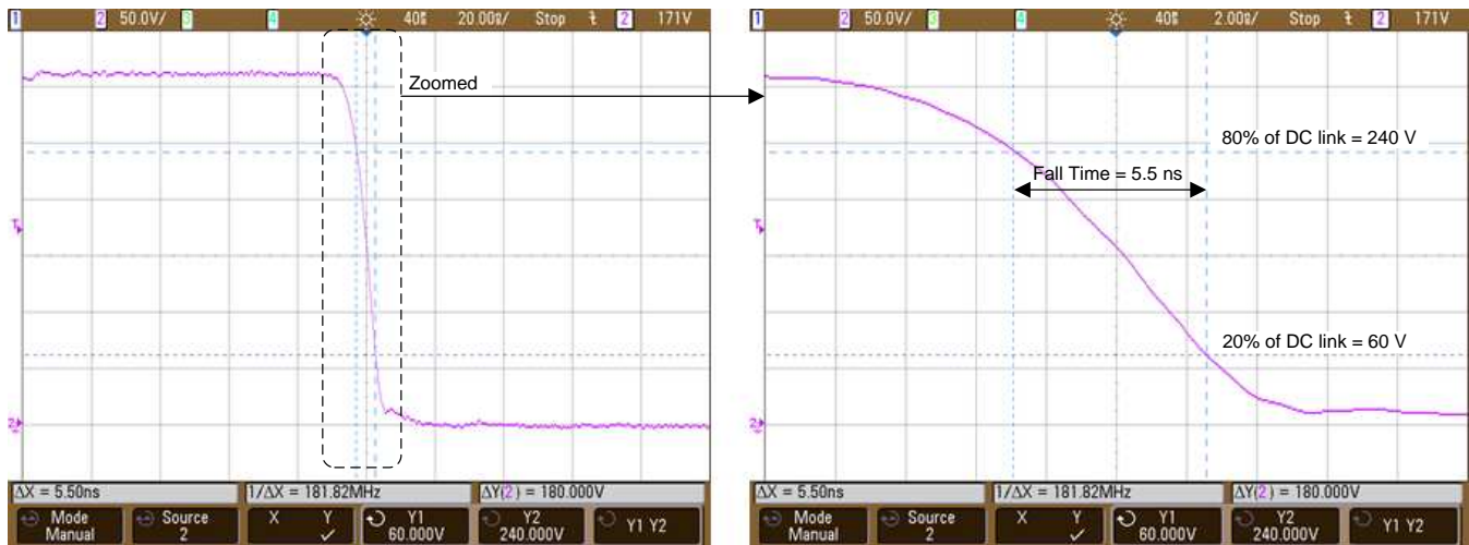
Figure 25. Turn-on Transition at 1.6 A
