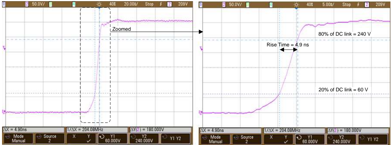
Figure 27. Turn-off Transition at 1.6 A
