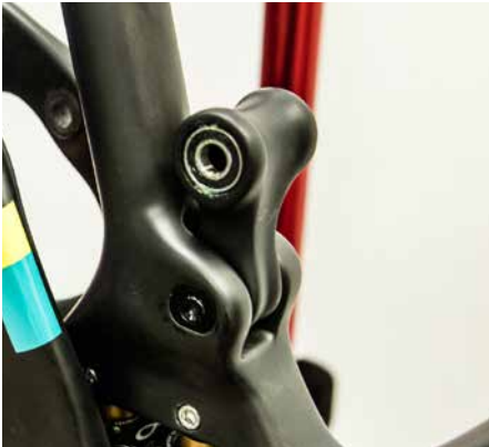
11. Your lower link pivot is now complete. Wipe any excess grease from the pivot axle area now and double check your torques. This is more difficult later in the process.
