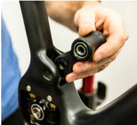
07. Insert the lower end of the link into the frame with the bearing race extending washers in place. Gently rest the link upright in the frame.
