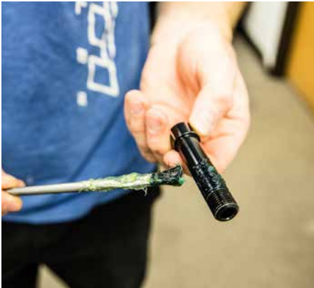
12. Grease the main pivot collet axle (300040485), including the threads.
