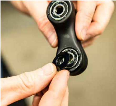
06. Place the bearing race extender washers (300020049) on the lower link bearings. There should be just enough grease there to hold the washers in place.
