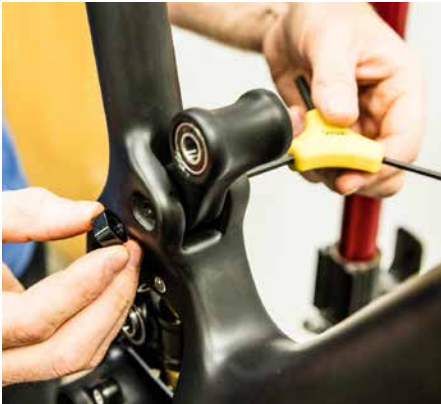
09. Insert the collet axle nut (300030287) in the corresponding keyed hole and thread the axle in using a 5mm allen wrench. This acts like a headset and is meant to preload the bearings.
