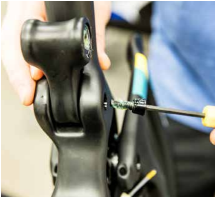
10. Grease and install the well greased lower link collet wedge. (300040486) Tighten with a 4mm allen wrench and finish with a torque wrench.
