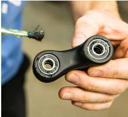
05. Lightly grease the bearing surfaces on your link.
