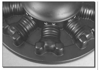
□ 8. Drill a 1/8" [3mm] hole into each of the crankcases as shown.
