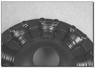
□ 7. Drill a 1/8" [3mm] hole into each of the cylinder heads as shown.
