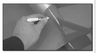
□ 2. When you are satisfied with the positioning, mark the outline of the fuselage onto the top and the bottom of the stabilizer with a fine point - felt tip pen.
