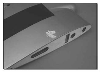
□ 5. On each outer rib of the center section there is a string taped. Remove the tape and re-apply the tape and string onto the top of the center section.
