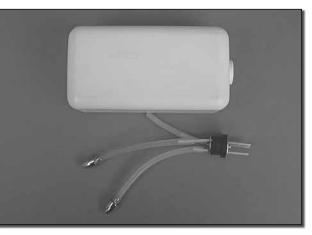
□ 4. Assemble the **fuel tank** as shown in the sketch. When tightening the center screw, be sure not to overtighten it. You just want it snug enough to pull the rubber stopper tight against the tank.
