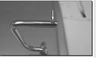
$\Box$   $\Box$  10.File a flat spot onto the end of the axle.
