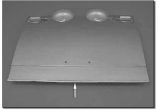
□ 12. Using the same technique used for the wing flaps, install four hinges into the flap of the wing **center section**.
