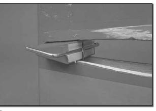
□ 10. Position the filler block in the back of the stab opening. Locate the joiner wire into the filler block as shown. Apply a couple of drops of oil to the wire as done with the flap hinges.
