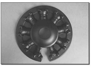
□ 6. Cut away the portion of the dummy engine that will be in front of the engine cylinder. This is needed for proper cooling of the engine. When determining the exact location to cut, note that cylinders should be oriented as shown in the picture. We were able to cool the O.S. .91 by only cutting away a small portion of the cylinders as shown in the picture.
