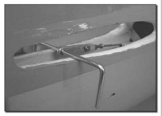
□ 9. Place the joiner wire into the stab opening and attach the clevis into the last hole in the arm of the joiner wire. Slide the silicone clevis keeper over the clevis.
