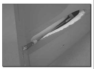
□ 8 Slide the end of the wire into the plastic tube at the stab opening in the fuselage.
