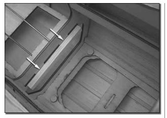
$\Box$  6. Locate the 6 x 6 x 90mm hardwood stick. Glue it in position on the fuselage former as shown. The stick should be glued on line with the visible tab slot.
