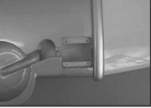
□ □ 3. Position the landing gear onto the landing gear rails as shown here. With a pencil or fine tip marker, mark the location of the holes for mounting the retracts.
