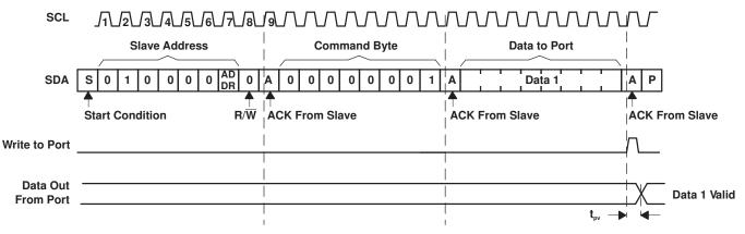
Figure 27. Write to Output Port Register
