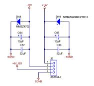
Figure 20. Front End Power Supply Connector and Filter
