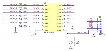
Figure 17. Digital Output Relay Driver
