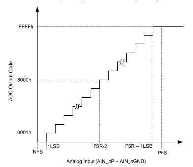
Figure 24. ADC Transfer Function
