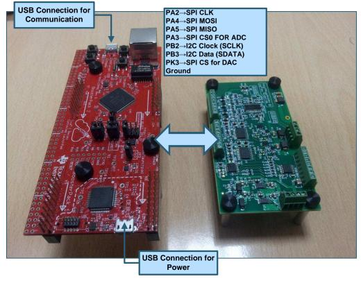
Figure 35. Connection With Host Controller
