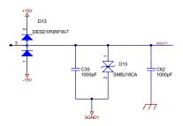
Figure 23. Analog Output EMC Protection
