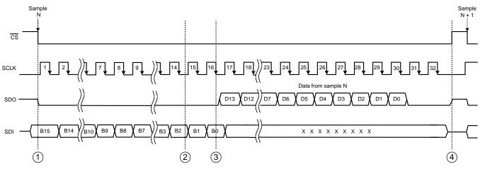
Figure 25. Device Operation Using the Serial Interface Timing Diagram of ADS8684
