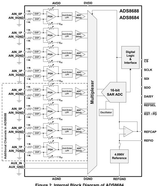
Figure 2. Internal Block Diagram of ADS8684
