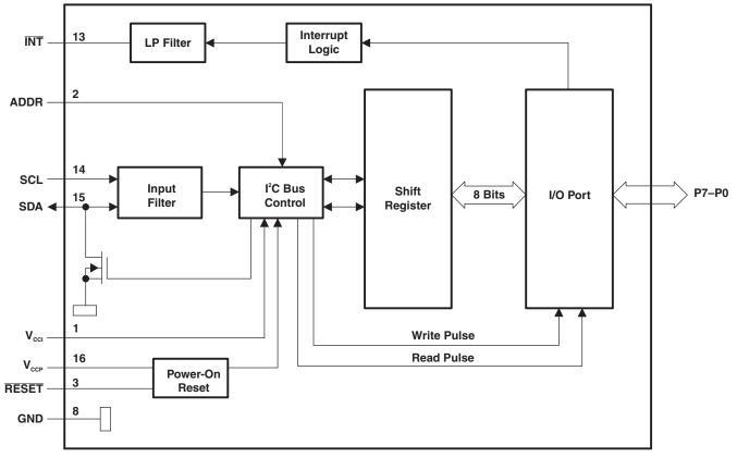
A All pin numbers shown are for the PW package. B. All I/Os are set to inputs at reset.
