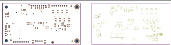
Figure 49. Bottom Solder Mask
