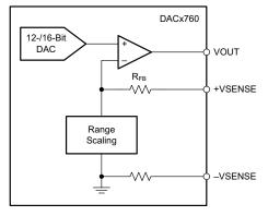
Figure 9. Voltage Output
