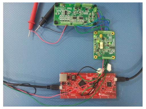
Figure 38. Interface With TIDA-00300 TI Design Board
