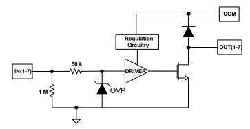
Figure 14. TPL7407L Functional Block Diagram
