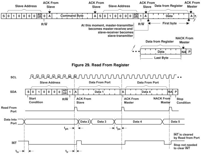
Figure 30. Read From Input Port Register
