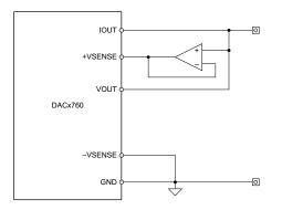
Figure 12. VOUT and IOUT Tied Together to One Terminal
