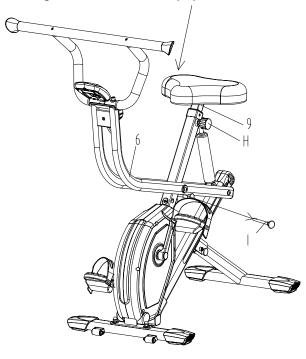
2. Hold the **Handle Bar Supporting Post (#6)** by the left hand, and grasp the **Saddle (#57)** by the right hand and push it forward until the oval-shaped holes on the **Handle Bar Supporting Post (#6)** and **Main Frame (#5)** align with each other. (Refer to the drawing No. A). Then insert **Pin (#I)**. (Refer to drawing No. B).
