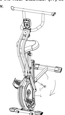
4. Align the two holes on the **Rear Stabilizer (#7)** and **Sliding Tube (#4)**. Insert **Pin (#L)** to finish this process.
