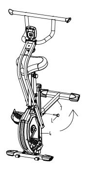
3. Hold the **Handle Bar Supporting Post** (#6) by the left hand, grasp the **Saddle** (#57), then press it downward till the **Rear Stabilizer** (#7) touches the ground.
