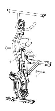
4. Insert the **Pin (#I)** into the **Handle Bar Supporting Post (#6)**.
