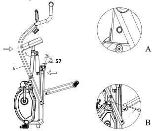
3. Hold the **Rear Stabilizer (#7)** by the right hand, pull **Pin (#L)** out first, then rotate the **Rear Stabilizer (#7)** as shown below.
