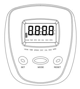
The meter turns on when you start pedaling or when you press a key. After 4 minutes of inactivity, the meter shuts off.
