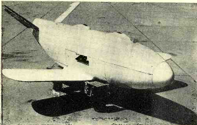
The "Gargoyle," an air-to-ground, radio-controlled powered glide bomb, carrying a standard 1000 lb. general-purpose or armor-piercing payload. It can be launched from airplanes.
