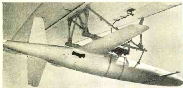
The TD2N-1, an air launched target, jet powered guided missile.
