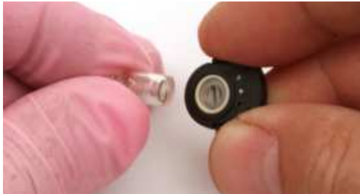
Figure 17: Reinstalling Electrode Lamp
