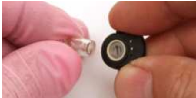
Figure 15: Reinstalling the Electrode Lamp
