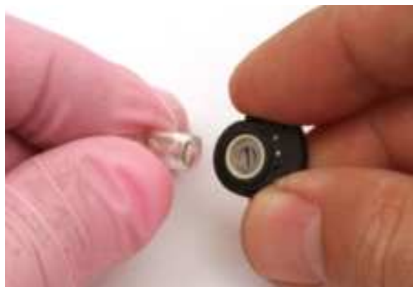
Figure 13: Reinstalling the Electrode Lamp
