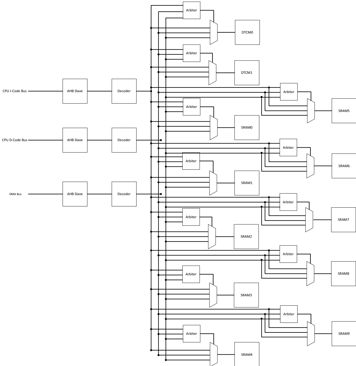
Figure 8. Block diagram for the SRAM Interface
