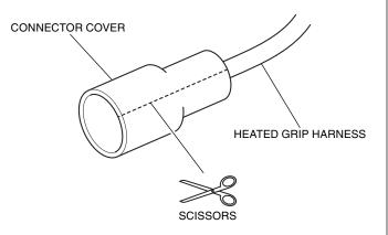
43. Remove the connector cover as shown.
