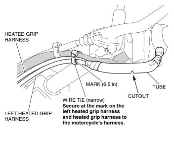
61. Secure the heated grip harness and left heated grip harness with the clamp as shown.
