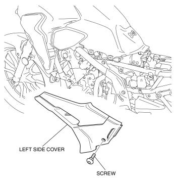
3. Remove the parts as shown.
