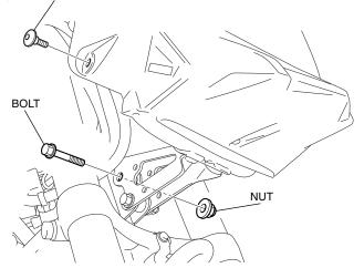
8. Loosen the nut and move the front upper cowl as shown.
