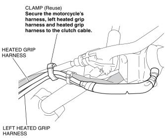
62. Secure the right heated grip harness with the wire ties as shown.
