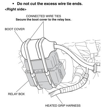
48. Secure the heated grip harness with the wire tie as shown.
