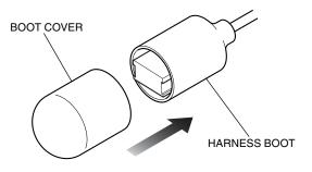
41. Secure the boot cover with electrical tape as shown.
