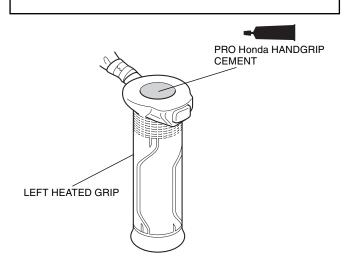
34. Apply Pro Honda Handgrip Cement to the left handlebar as shown.
