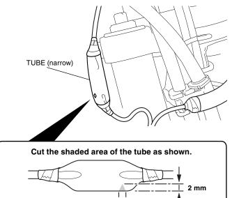
55. Secure the heated grip harness behind the throttle cable as shown.
