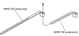
47. Secure the boot cover with the wire ties as shown.
