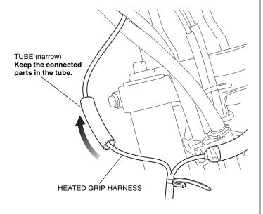
53. Secure the tube with electrical tape as shown.
