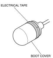
42. Cut the connector cover as shown.
