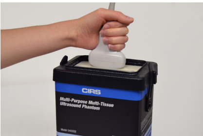
Water well for coupling curved probes
