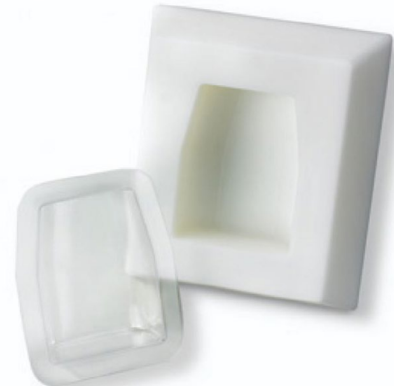
Thermoformed packaging cover and FDM mold.
