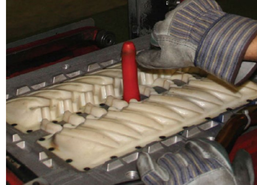
Matchplate with FDM insert in molding machine.
